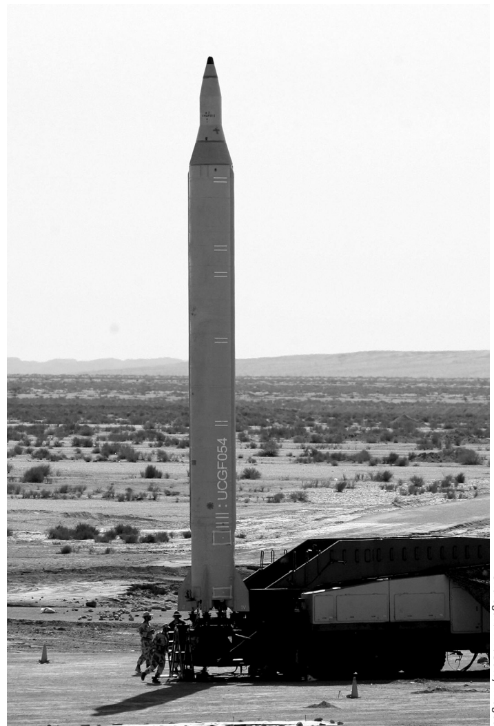
An Iranian Ghadr-1 medium-range ballistic missile (MRBM) is prepared for a flight test in September 2009. This single-stage, liquid-fueled derivative of the Shahab-3 MRBM could deliver a 750-kilogram payload some 1,600 kilometers. The Ghadr-1 is the most capable MRBM in Iran's operational inventory and would be suitable for delivering a nuclear weapon.
